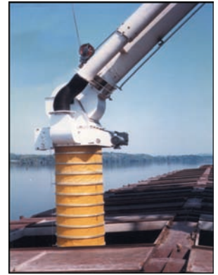
Pivoting gimbal allows different loading angles.
