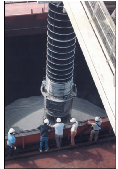
Dust free dry phosphate loading into ships.
