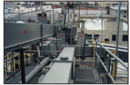
Aeration conveyors distributing to multiple silos using a combination of turning boxes and vertical slide gates.
