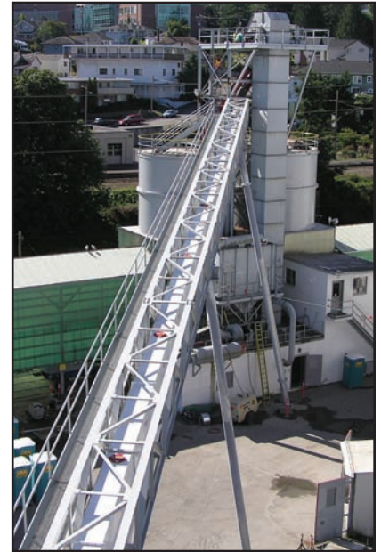
Aeration conveyor being fed by bucket elevator.
