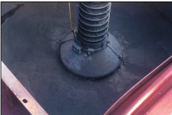
Loading aerated cement into barges dust free using "H-Style Deadfall".
